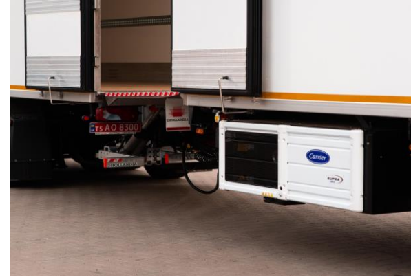
Refrigeration and heating unit for the trailer
